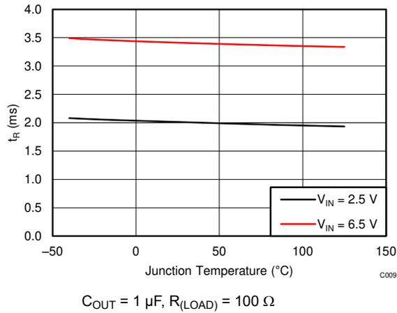
图 7-13. Output Rise Time ( $t_R$ ) vs Temperature
