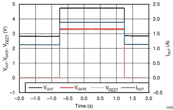
图 9-14. Two-Level Current Limit With  $R_{LOAD} = 2.5 \Omega$
