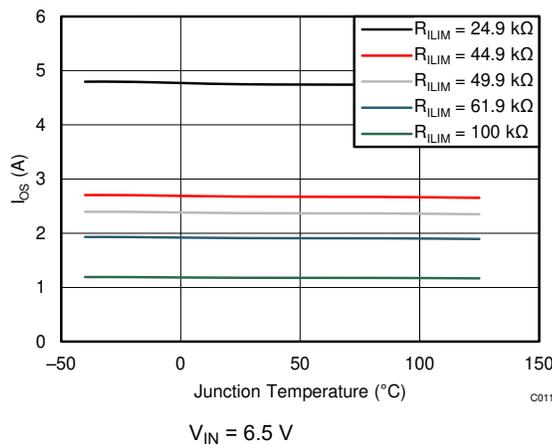
图 7-15. Short-Circuit Current ( $I_{OS}$ ) vs Temperature
