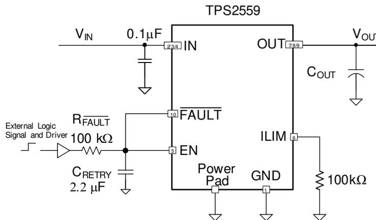
图 9-4. Auto-Retry Circuit with External EN Signal
