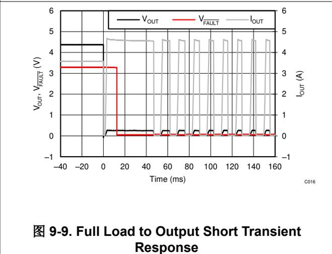
图 9-9. Full Load to Output Short Transient Response
