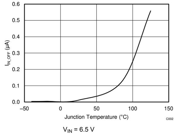
图 7-6. Supply Current, Output Disabled ( $I_{IN\_OFF}$ ) vs Temperature
