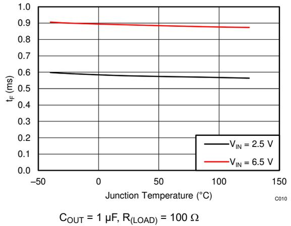
图 7-14. Output Fall Time ( $t_F$ ) vs Temperature
