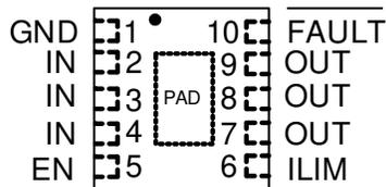
图 6-1. DRC Package, 10-Pin VSON, Top View
