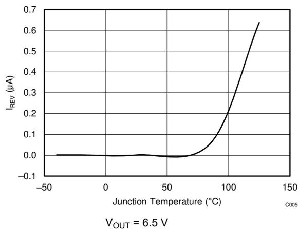
图 7-9. Reverse Leakage Current ( $I_{REV}$ ) vs Temperature
