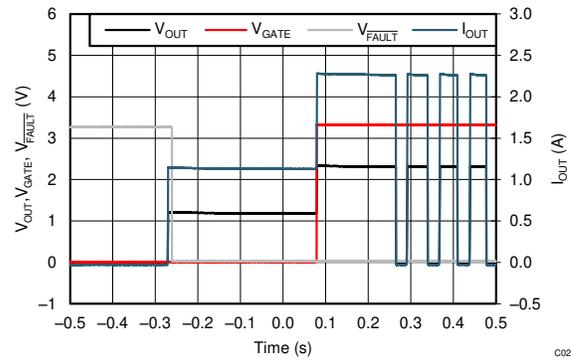
图 9-15. Two-Level Current Limit With  $R_{LOAD} = 1 \Omega$
