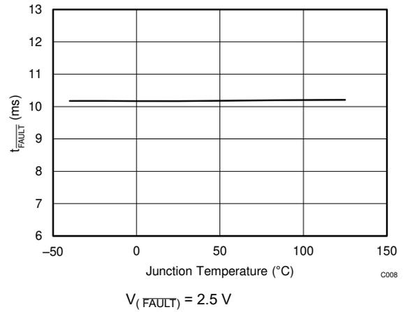
图 7-12. Deglitch Time ( $t_{FAULT}$ ) vs Temperature
