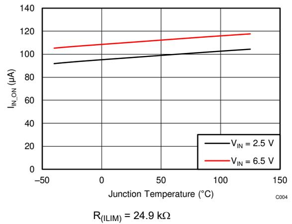
图 7-8. Supply Current, Output Enabled ( $I_{IN\_ON}$ ) vs Temperature
