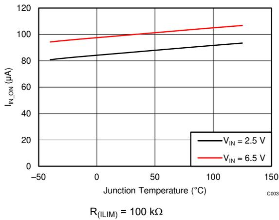
图 7-7. Supply Current, Output Enabled ( $I_{IN\_ON}$ ) vs Temperature
