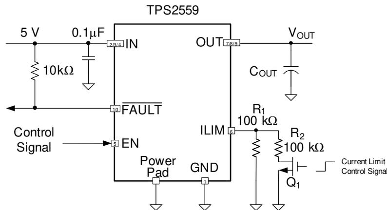
图 9-5. Two-Level Current-Limit Circuit
