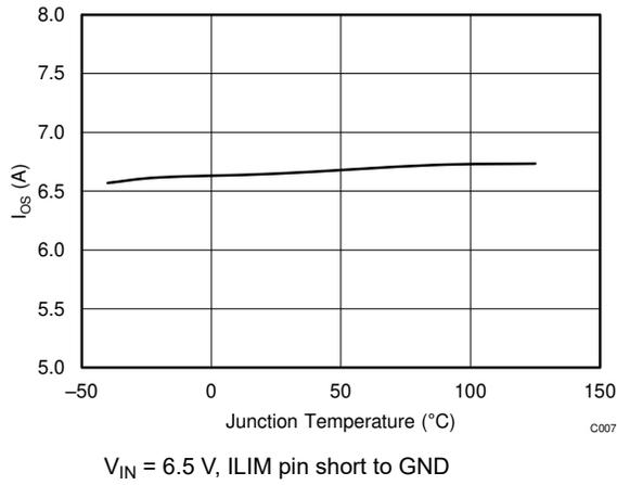
图 7-11. Short-Circuit Current ( $I_{OS}$ ) vs Temperature
