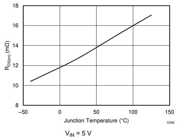
图 7-10. Input/Output Resistance ( $R_{DS(on)}$ ) vs Temperature
