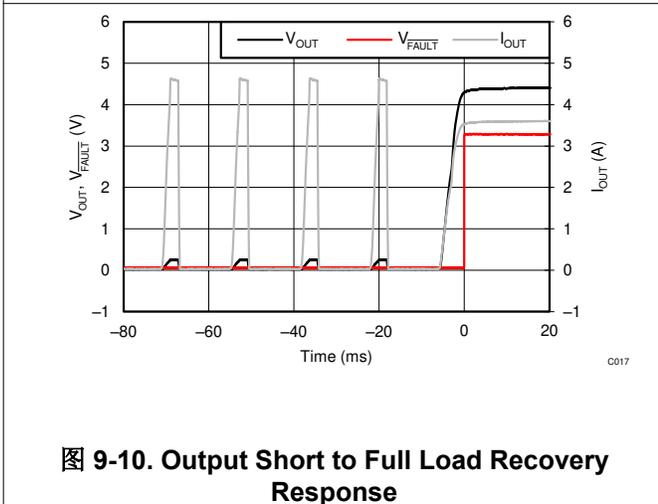
图 9-10. Output Short to Full Load Recovery Response
