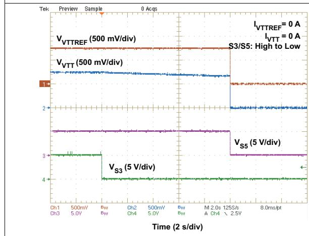
图 21. Shutdown Waveforms (S3/ S5: High to Low)
