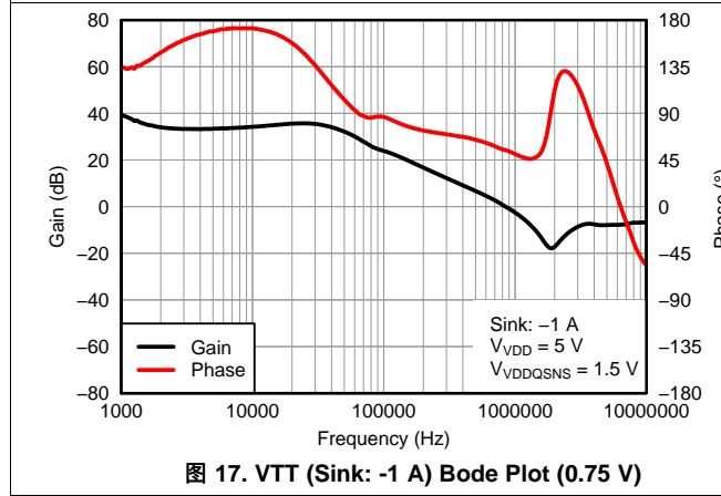
图 17. VTT (Sink: -1 A) Bode Plot (0.75 V)
