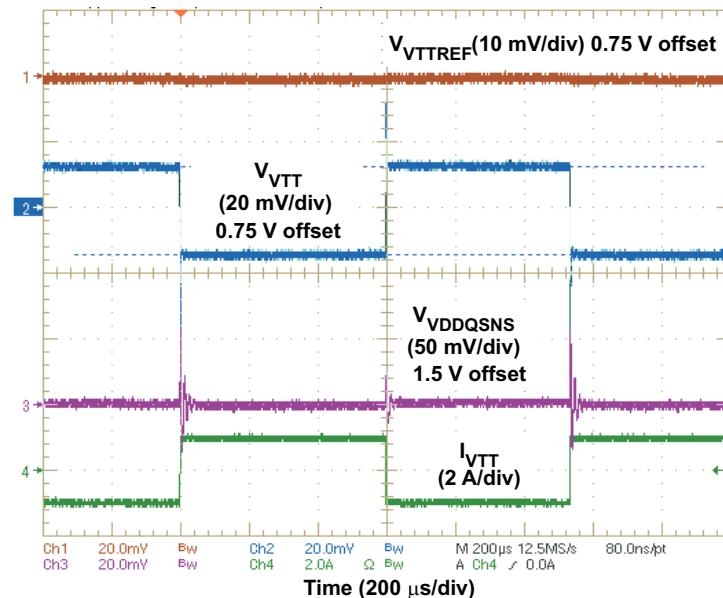
**图 26. VTT Load Transient Response (0.75 V)**
