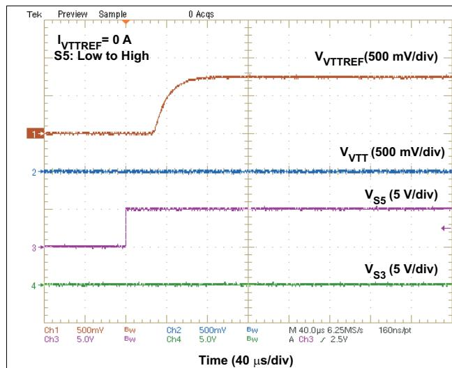
图 19. Start-Up Waveforms (S5: Low to High)
