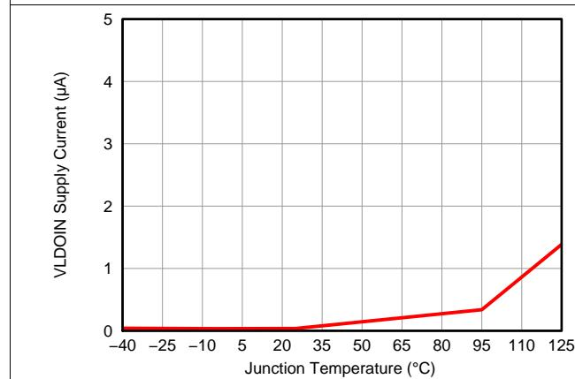
图 3. VLDOIN Supply Current vs. Junction Temperature
