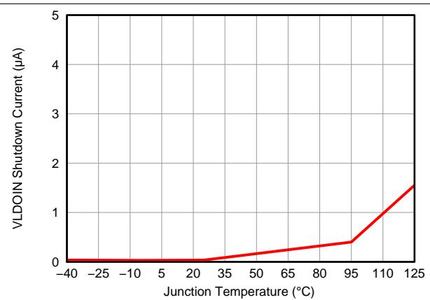
图 4. VLDOIN Shutdown Current vs. Junction Temperature
