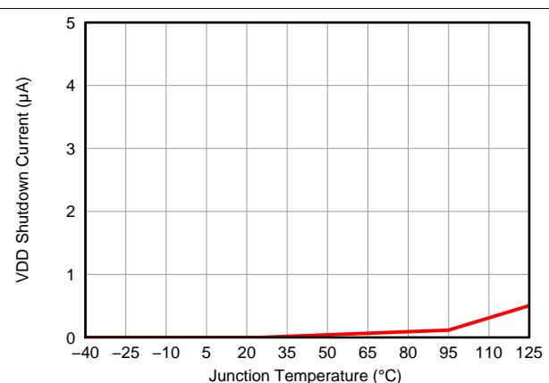
图 2. VDD Shutdown Current vs. Junction Temperature
