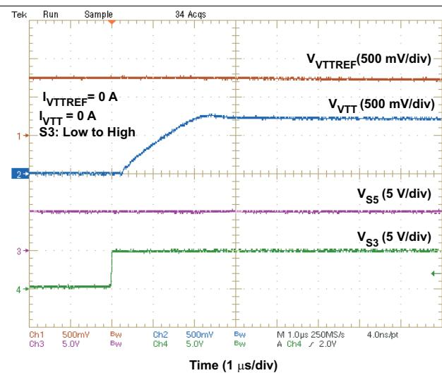
图 20. Start-Up Waveforms (S3: Low to High)
