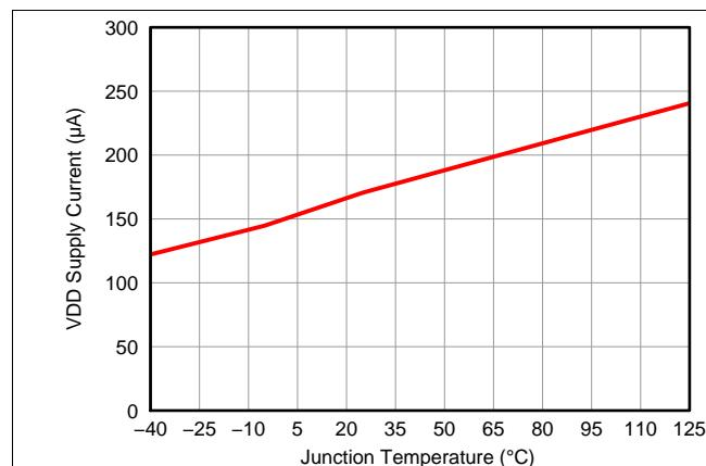
图 1. VDD Supply Current vs. Junction Temperature
