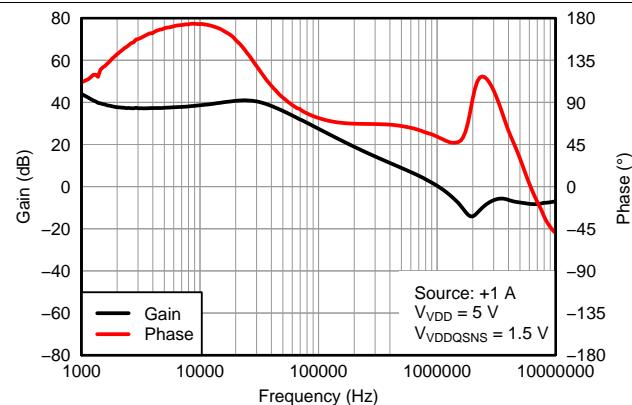
图 18. VTT (Source: +1 A) Bode Plot (0.75 V)
