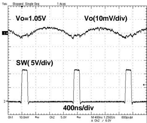
**Figure 13. VOLTAGE RIPPLE AT OUTPUT (Io = 6 A)**
