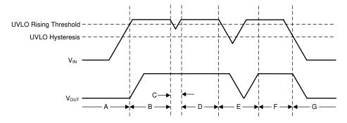
图 45. Typical UVLO Operation
