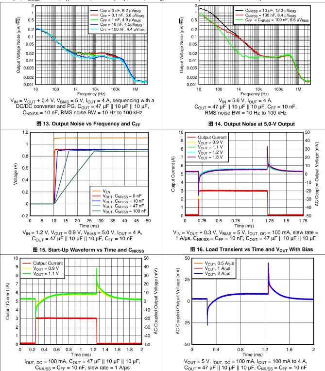
图 17. Load Transient vs Time and V<sub>OUT</sub> Without Bias
