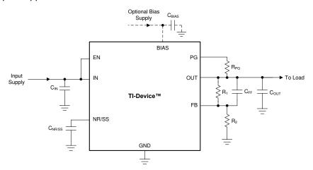
图 54. Typical Application for a 0.9-V Rail
