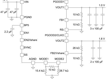
图 8-1. TPSM5D1806 Dual Output Typical Schematic
