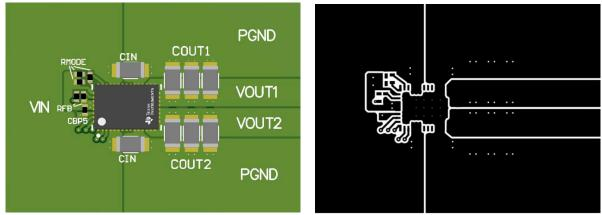
图 10-1. Typical Dual-Output Layout
