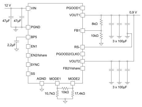
图 8-2. TPSM5D1806 Parallel Outputs Typical Schematic
