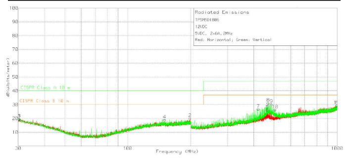
图 10-4. Radiated Emissions 12-V Input, 5-V Output, 6-A/Output Load
