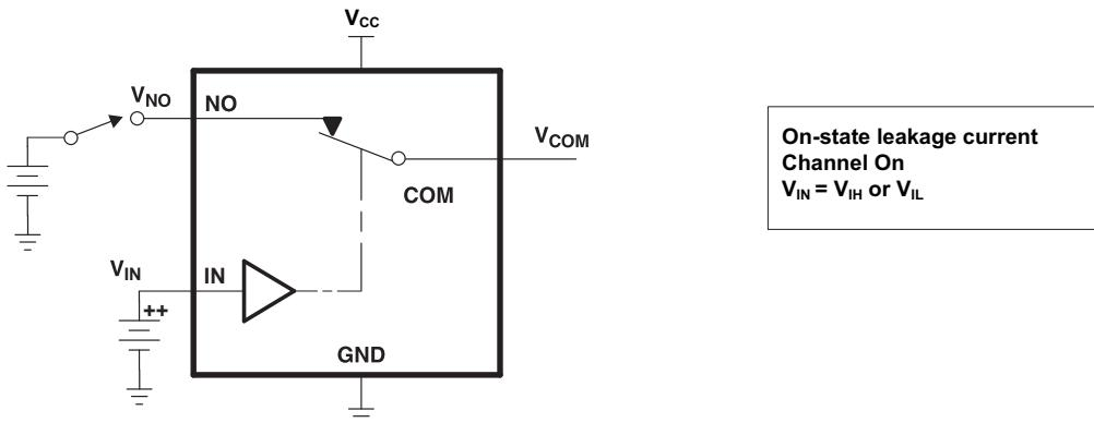
**Figure 15. ON-state leakage current
