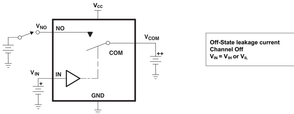
**Figure 14. OFF-state leakage current ( $I_{COM(OFF)}$ ,  $I_{NO(OFF)}$ )**
