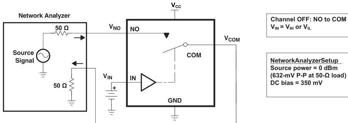
**Figure 20. OFF isolation (O<sub>ISO</sub>)**
