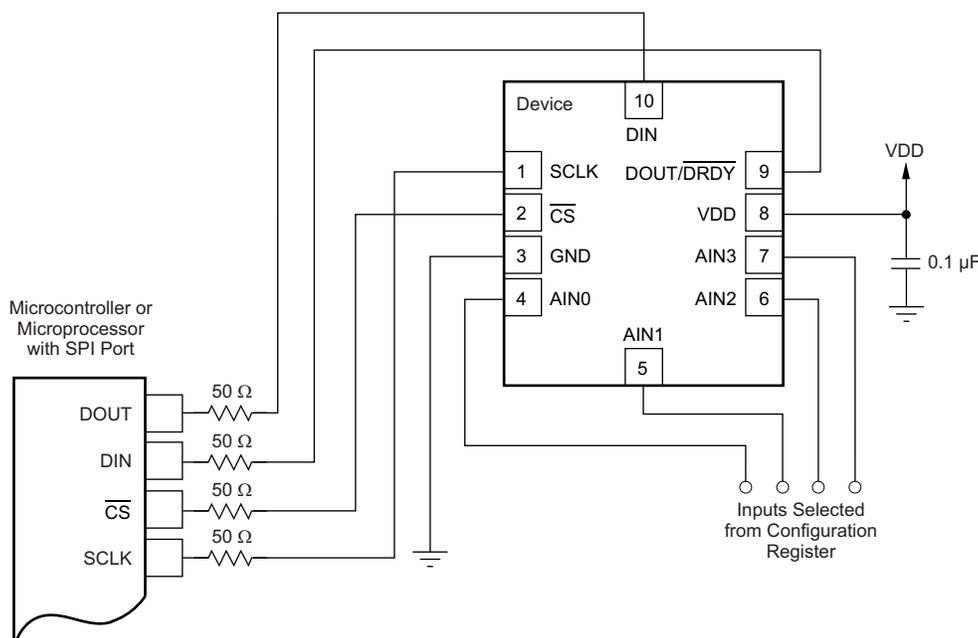
**Figure 18. Typical Connections**
