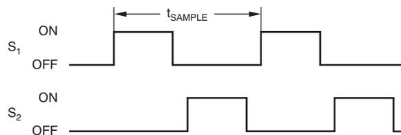
Figure 10. S<sub>1</sub> and S<sub>2</sub> Switch Timing
