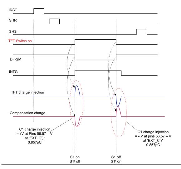
图 9. TFT Charge Injection Compensation Scheme
