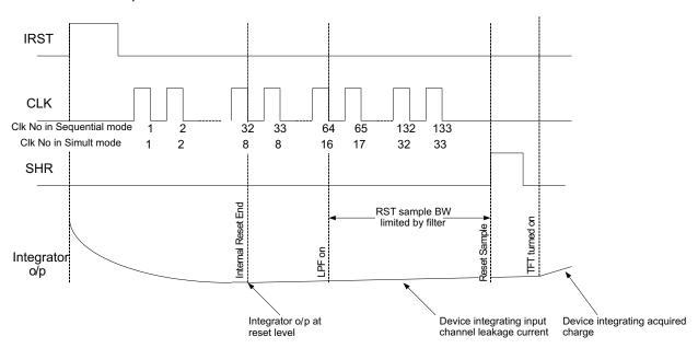
图 3. Timing Diagram Showing Details of Reset Phase
