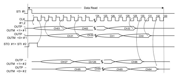
图 8. Data Read with Two Devices in Cascade
