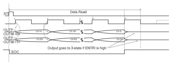
图 6. Device Data Read in Simultaneous Mode (SMT MD=1)
