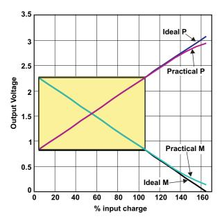
The plot above shows AFE transfer characteristics in integrator down mode. (For integrator up mode the P and M plots are interchanged.) AFE output is linear in the charge range bound by the rectangle shown.
