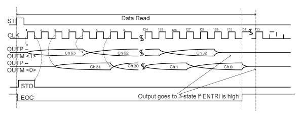
图 5. Device Data Read in Sequential Mode (SMT\_MD = 0)
