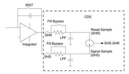
图 1. Integrator Channel Schematic
