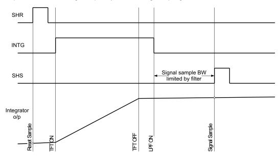
图 4. Timing Diagram Showing Details of Integration Phase
