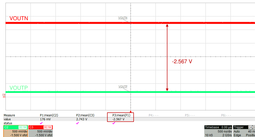
图 6-5. Typical Fail-Safe Output of the AMC3330
