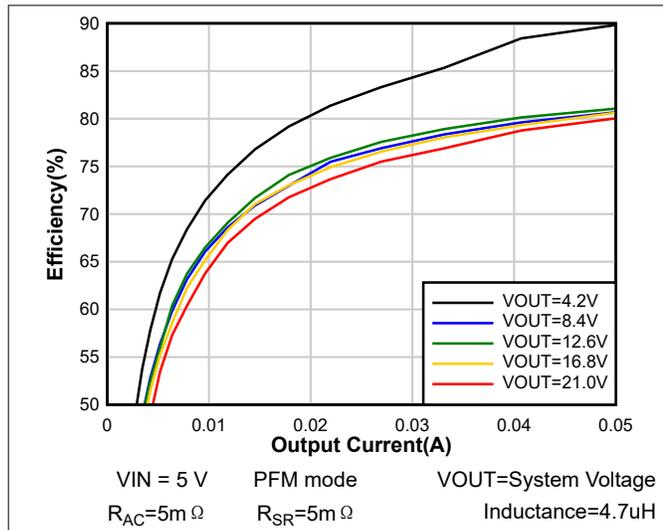
图 7-1. Light Load System Efficiency
