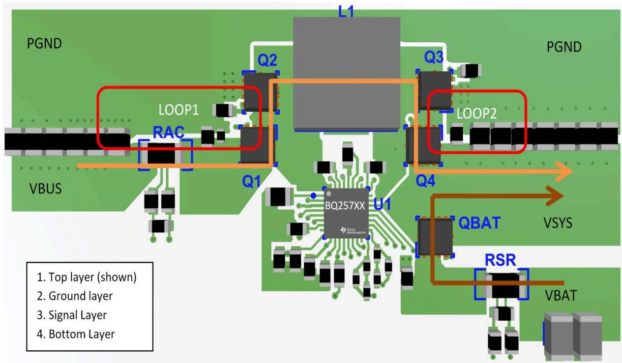
图 11-1. Buck-Boost Charger Layout Reference Example Top View
