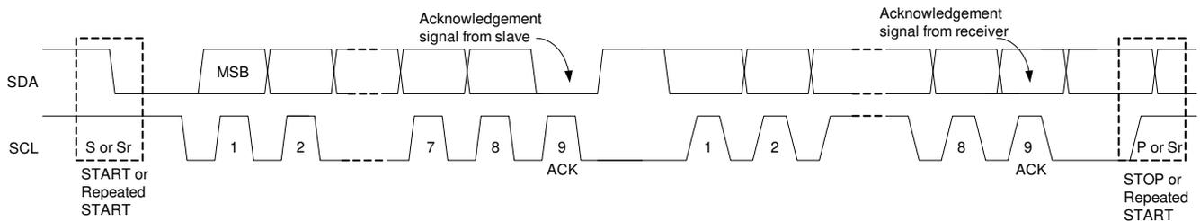
图 8-10. Data Transfer on the I<sup>2</sup>C Bus
