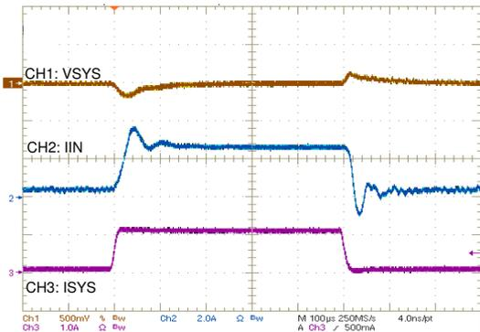
VBUS = 5 V/3.25 A, 3-cell, VSYS = 9 V, Without battery
