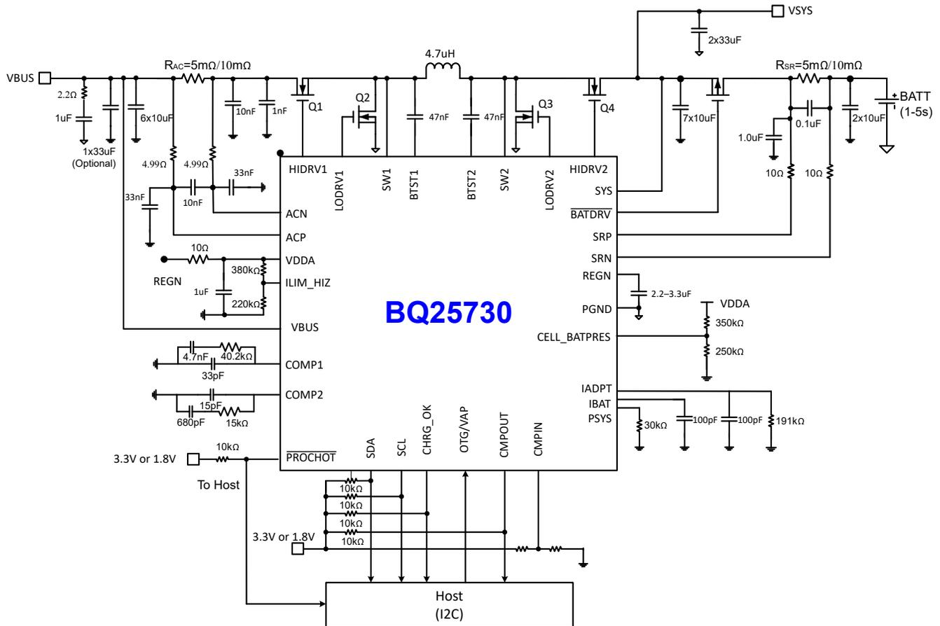
图 9-1. Application Diagram of BQ25730 with Power Path
