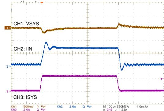
VBUS = 9 V/3.25 A, 3-cell, VSYS = 9 V, Without battery
