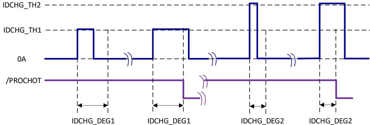
图 8-1. Two-Level Battery Discharging Current Trigger PROCHOT Diagram
