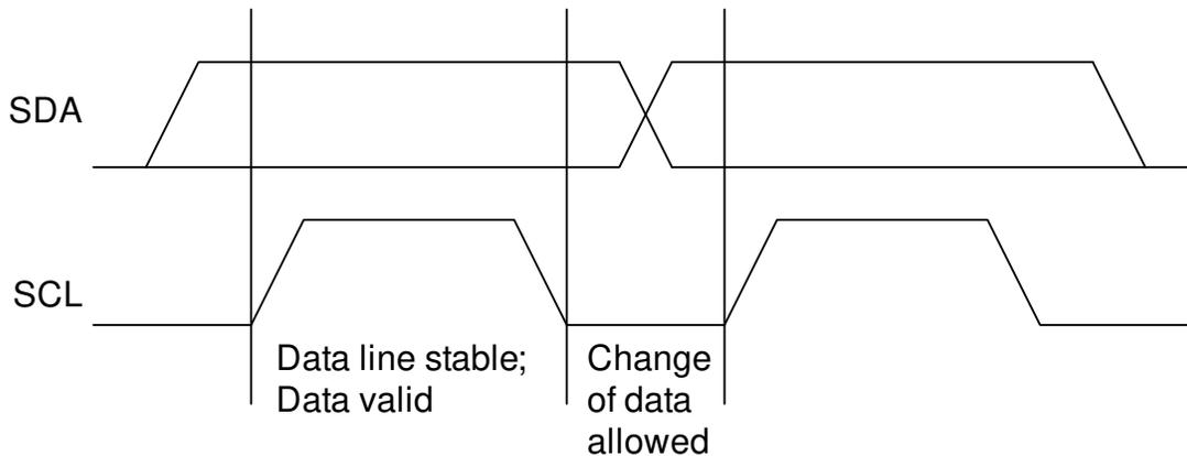
**图 8-8. Bit Transfer on the I<sup>2</sup>C Bus**
