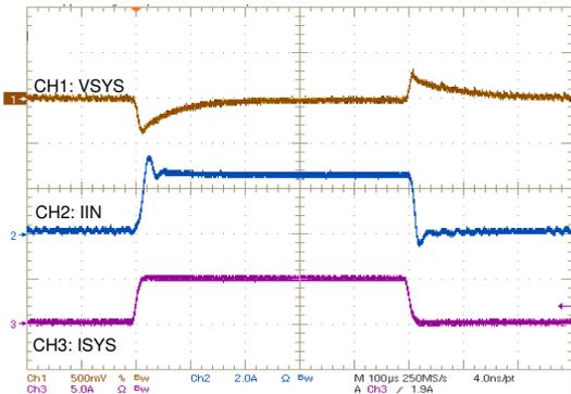
VBUS = 12 V/3.25 A, 3-cell, VSYS = 9 V, Without battery
