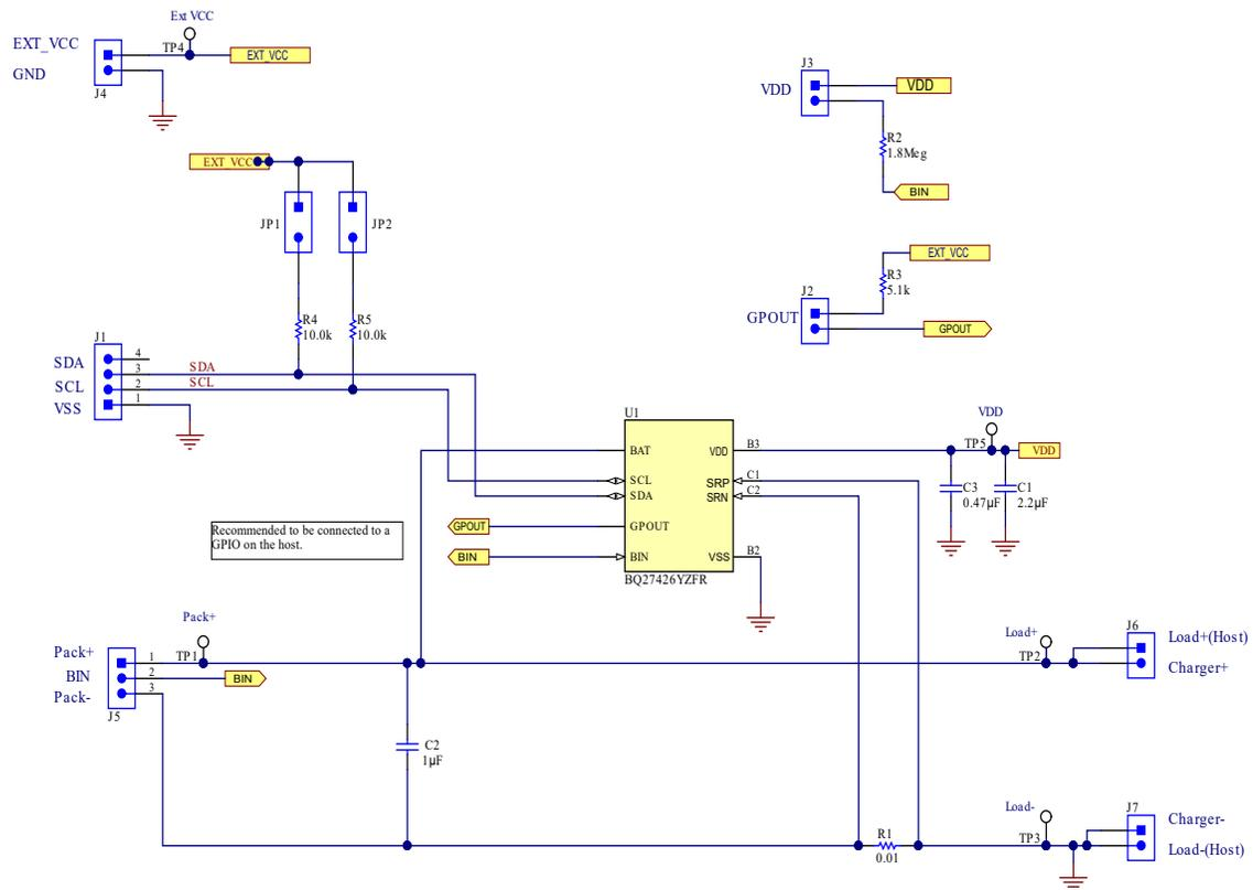
图 8-2. Typical Application with Low-Side Current Sense Resistor
