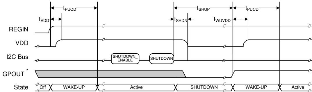
\* GPOUT is configured as an input for wake-up signaling.
