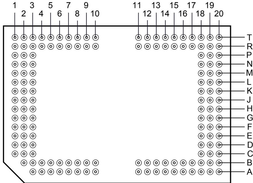
图 5-1. FYN Package 149-Pin PGA Bottom View
