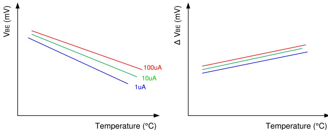
**图 7-3. Example of Delta VBE Versus Temperature**
