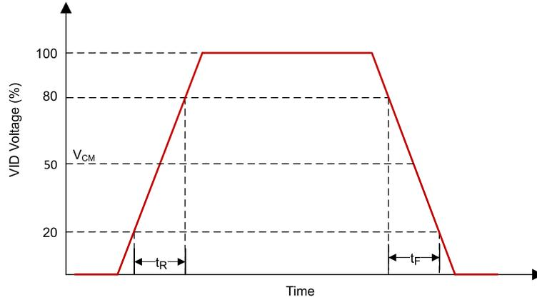
图 6-3. SubLVDS Input Rise and Fall Slew Rate
