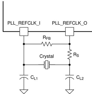
$C_L$  = Crystal load capacitance (farads)
