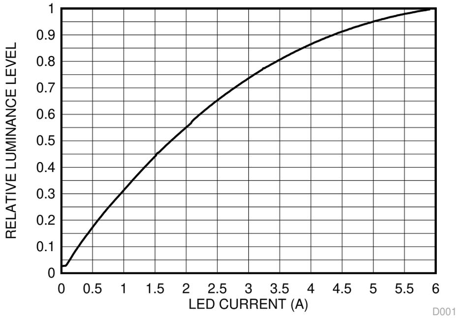
图 8-2. Typical Luminance vs Current
