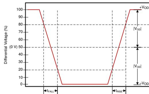
V<sub>CM</sub> is removed when the signals are viewed differentially
