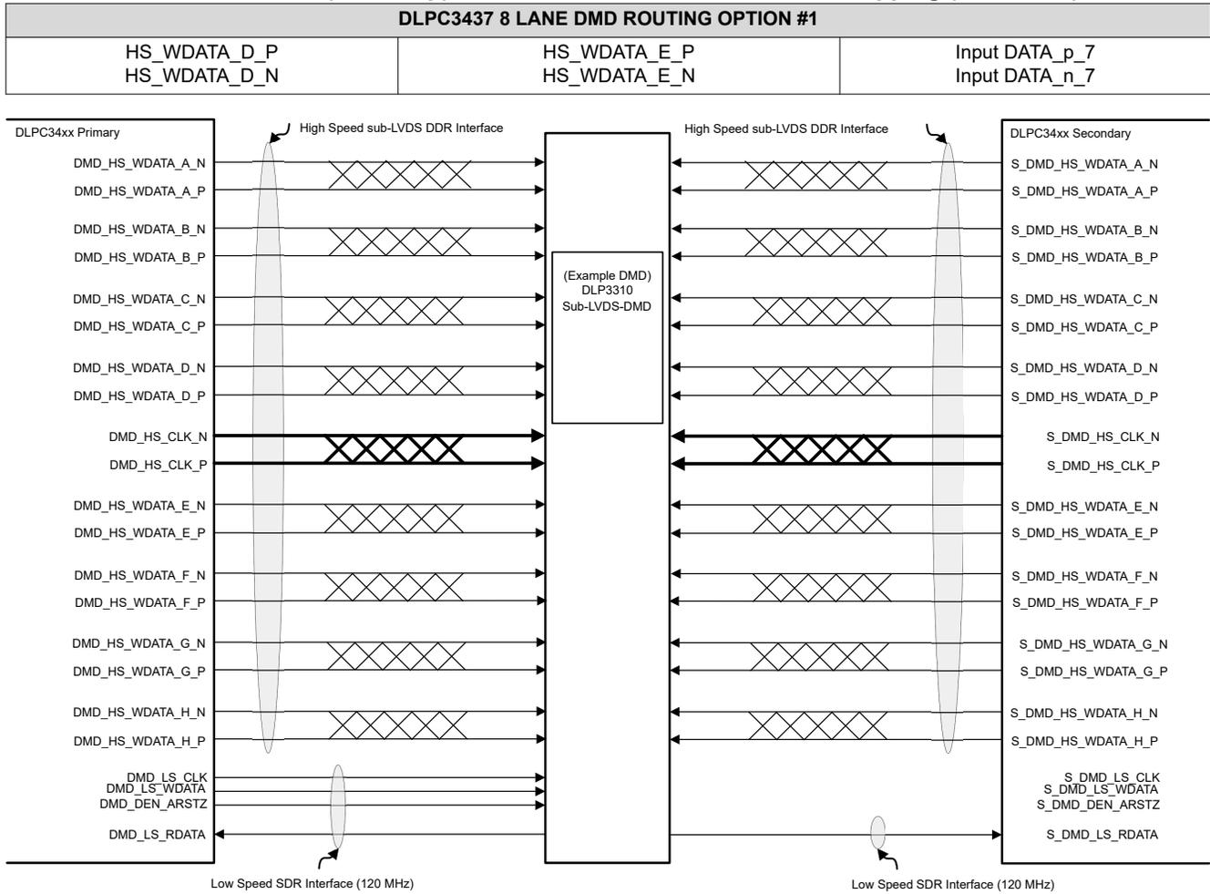
图 7-12. DLP3310 (.33 1080p) DMD Interface Example (Option 1 and 2)
