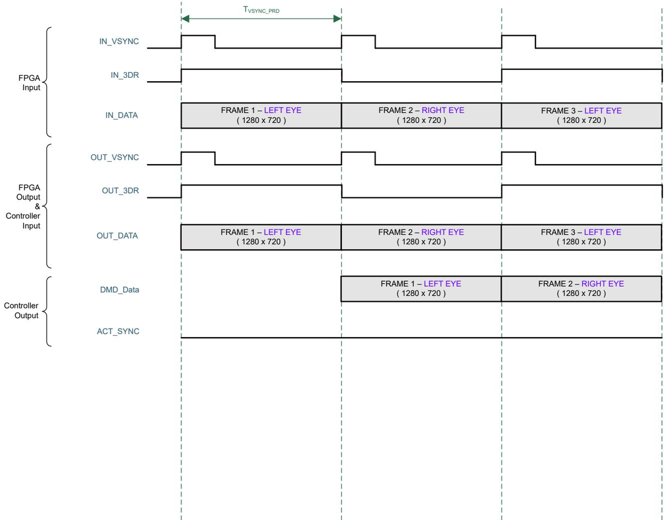
**图 7-3. DLPC3437 3D Frame and Signal Timing**
