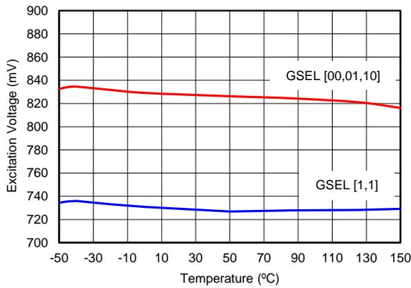
Figure 3. HALL SENSOR EXCITATION VOLTAGE vs TEMPERATURE
