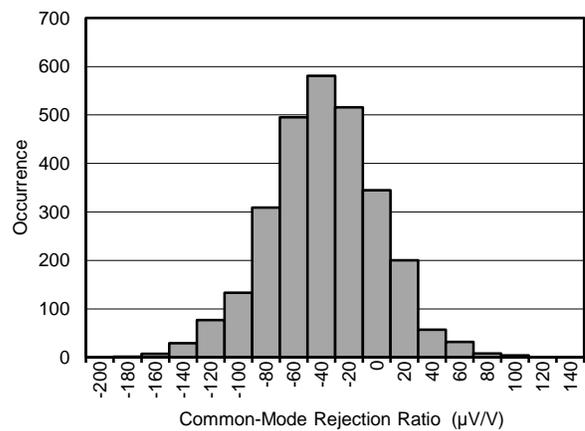
**Figure 18. DIFFERENTIAL AMPLIFIER COMMON-MODE REJECTION RATIO HISTOGRAM**
