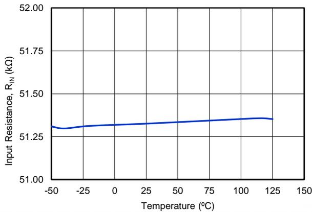
**Figure 21. DIFFERENTIAL AMPLIFIER REFERENCE INPUT IMPEDANCE vs TEMPERATURE**
