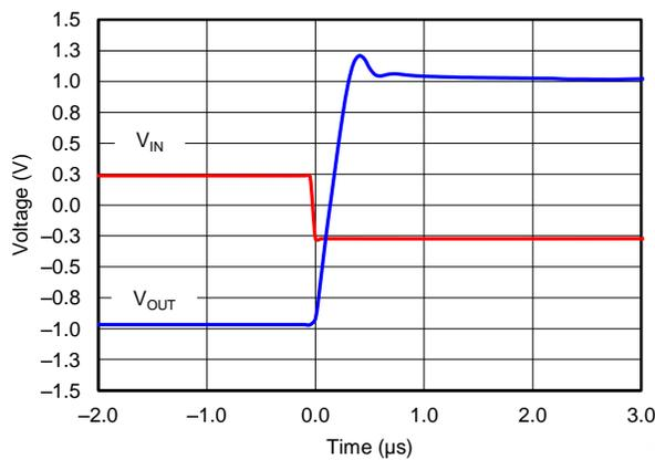
**Figure 35. DIFFERENTIAL AMPLIFIER SETTLING TIME (FALLING EDGE)**
