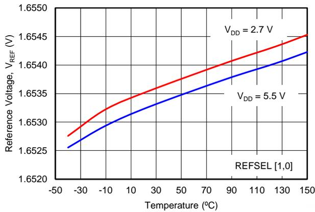
**Figure 43. 1.65-V REFERENCE OUTPUT VOLTAGE vs TEMPERATURE**
