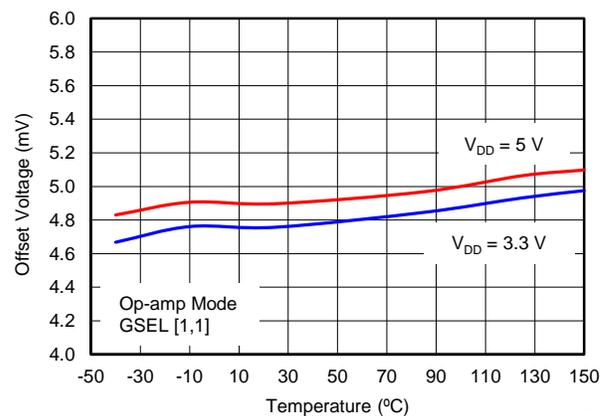
**Figure 12. FRONT-END OFFSET VOLTAGE vs TEMPERATURE (OP-AMP MODE)**
