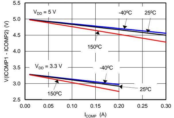
**Figure 14. OUTPUT VOLTAGE SWING vs POSITIVE OUTPUT CURRENT**
