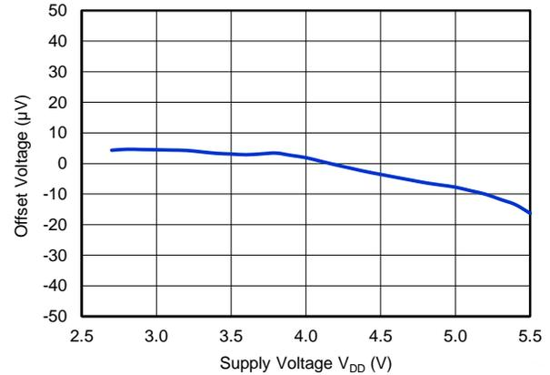
**Figure 20. DIFFERENTIAL AMPLIFIER OFFSET VOLTAGE vs POWER SUPPLY**
