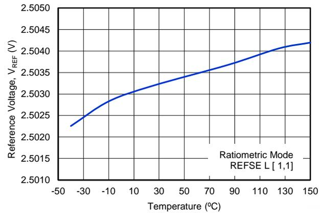
**Figure 44. RATIOMETRIC REFERENCE OUTPUT VOLTAGE vs TEMPERATURE**
