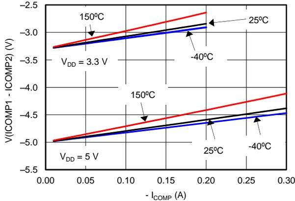
**Figure 13. OUTPUT VOLTAGE SWING vs NEGATIVE OUTPUT CURRENT**
