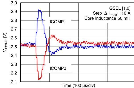
**Figure 51. Settling of ICOMP1 and ICOMP2 (Mode Gain\_3)**
