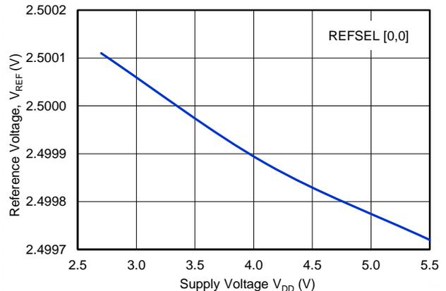
**Figure 40. 2.5-V REFERENCE OUTPUT VOLTAGE vs POWER SUPPLY**
