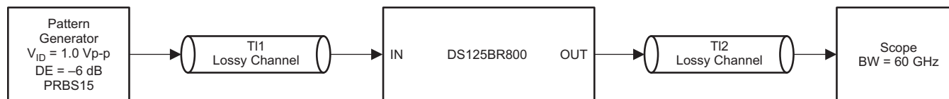
Figure 11. Test Setup Connections Diagram
