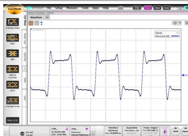
Figure 9-6. DS250DF230 FIR Transmit Equalization While Operating at 25.78125 Gbps
