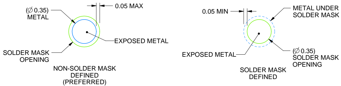
SOLDER MASK DETAILS NOT TO SCALE
