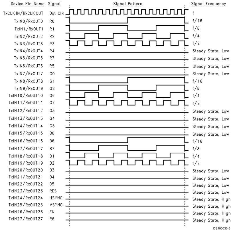
FIGURE 2. "16 Grayscale" Test Pattern (Notes 5, 6, 7, 8)
