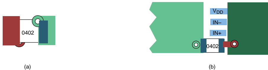
Figure 30. Typical Decoupling Capacitor Layouts
