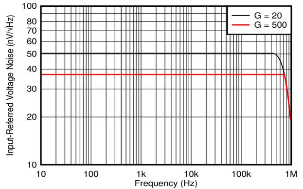
图 6-16. Input Referred Noise vs Frequency
