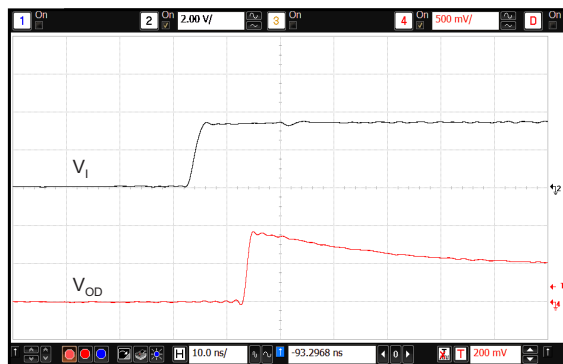
Figure 15. Distortion Correction Scheme Calibration Time ( t_{CALIB} )
