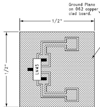
Printed Circuit Board Used for Heat Sink to Generate All Curves.
