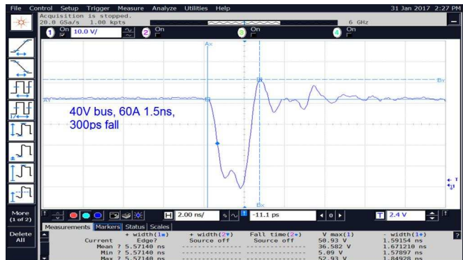
图 14. V_{DS} for 1.5 ns Pulse With 40V of Bus Voltage
