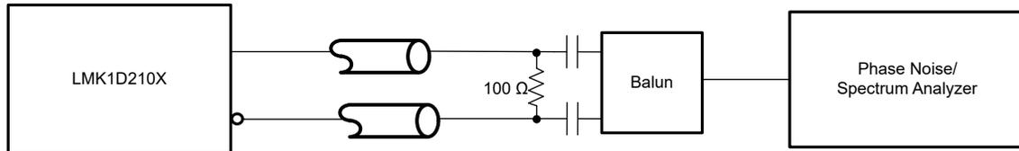
图 8-2. LVDS Output AC Configuration During Device Test
