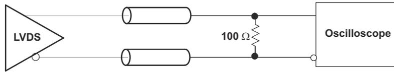
图 8-1. LVDS Output DC Configuration During Device Test
