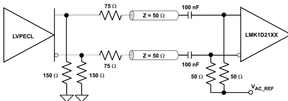
图 9-5. LVPECL Clock Driver Connected to LMK1D210x Input
