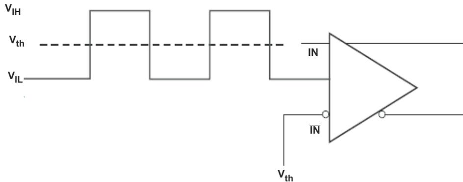
图 8-3. DC-Coupled LVCMOS Input During Device Test
