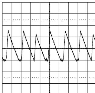
The inductor internal to the module is 10  $\mu H$ . This value was chosen as a good balance between low and high input voltage applications. The main parameter affected by the inductor is the amplitude of the inductor ripple current ( $I_{LR}$ ).  $I_{LR}$  can be calculated with:
