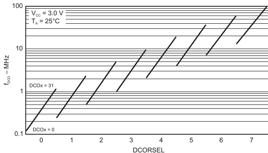
Figure 5-11. Typical DCO Frequency
