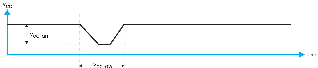
Figure 22. Glitch Width and Glitch Height
