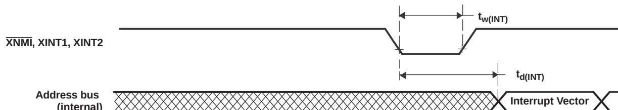
Figure 6-17. External Interrupt Timing
