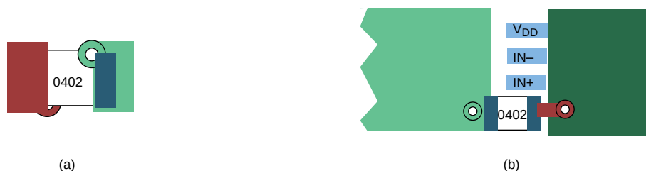
Figure 29. Typical Decoupling Capacitor Layouts
