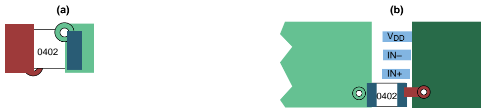
图 29. Typical Decoupling Capacitor Layouts
