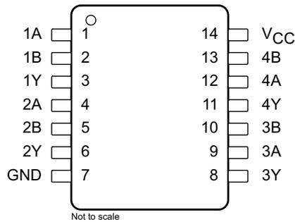
**Figure 5-1. D, DB, N, NS, J, W, or PW Package
