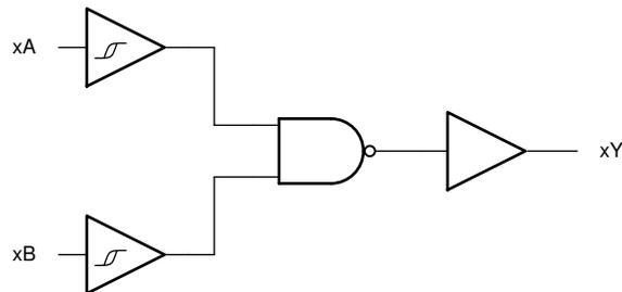
Figure 8-1. Logic Diagram (Positive Logic) for the SN74HC132
