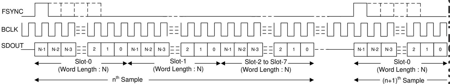
图 7-5. TDM 模式协议时序 (PASI\_TX\_OFFSET = 0 且 PASI\_BCLK\_POL = 1)
