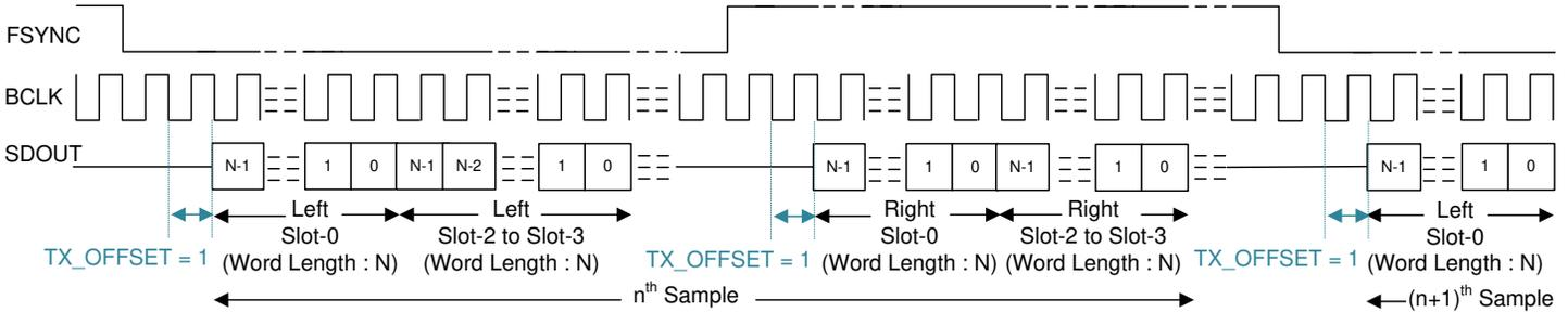
图 7-7. I²S 协议时序 (PASI\_TX\_OFFSET = 1)
