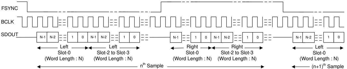
图 7-9. I²S 协议时序 (PASI\_TX\_OFFSET = 0 且 PASI\_BCLK\_POL = 1)
