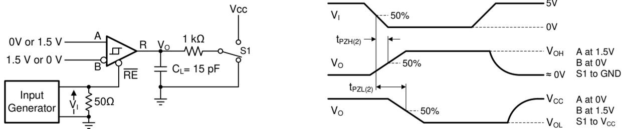
**图 16. Measurement of Receiver Enable Times With Driver Disabled**
