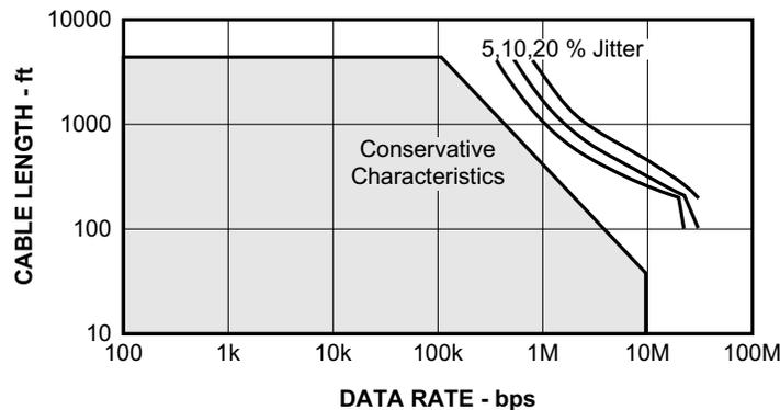
图 23. Cable Length vs Data Rate Characteristic
