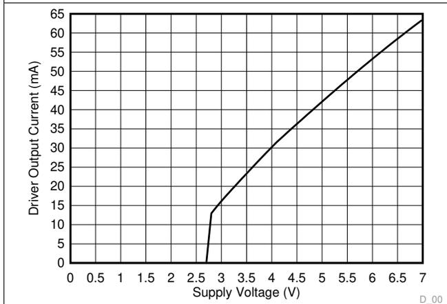
图 3. Driver Output Current vs Supply Voltage
