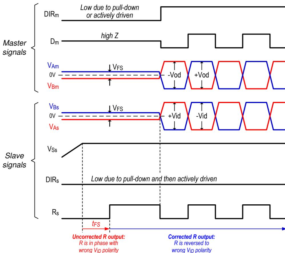
图 19. Polarity Correction Timing With Passive Polarity Definition
