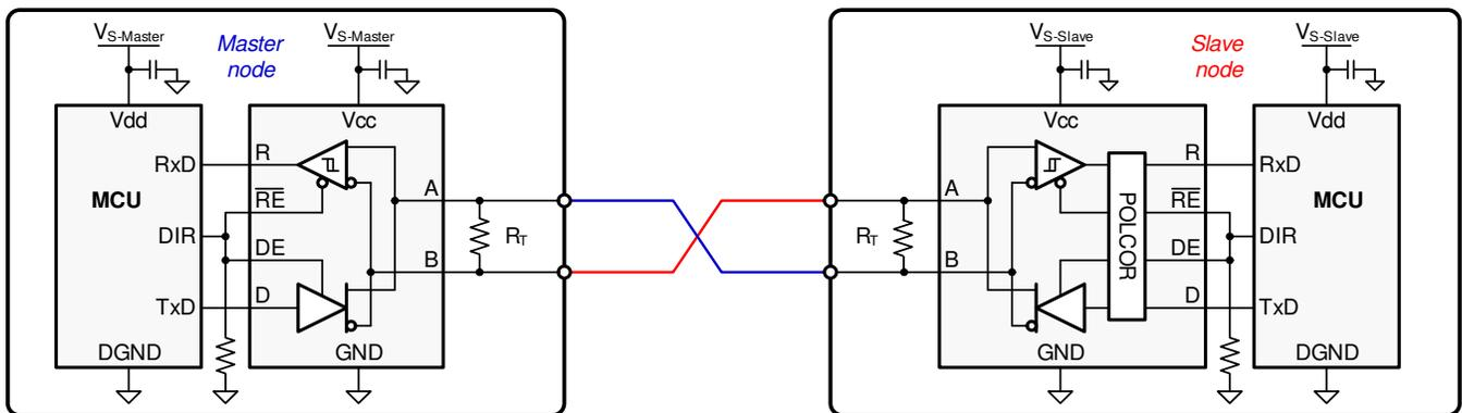
图 20. Active Polarity Definition
