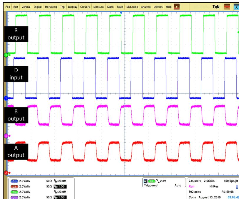
图 31. Waveforms at 1 Mbps Operation, Clock Data Pattern
