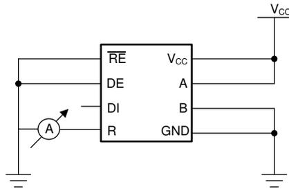
图 13. Measurement of Receiver Output Short Circuit Current
