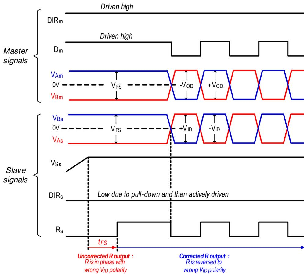
图 21. Polarity Correction Timing With Active Polarity Definition
