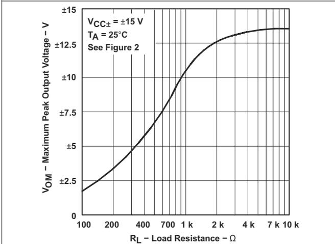
图 6-3. Maximum Peak Output Voltage vs Load Resistance
