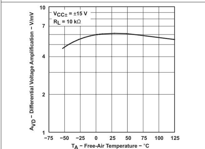
图 6-5. Differential Voltage Amplification vs Free-Air Temperature
