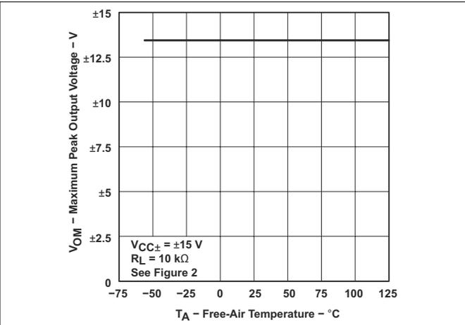
图 6-2. Maximum Peak Output Voltage vs Free-Air Temperature
