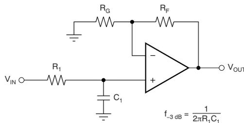
$$f_{-3\text{dB}} = \frac{1}{2\pi R_1 C_1}$$
