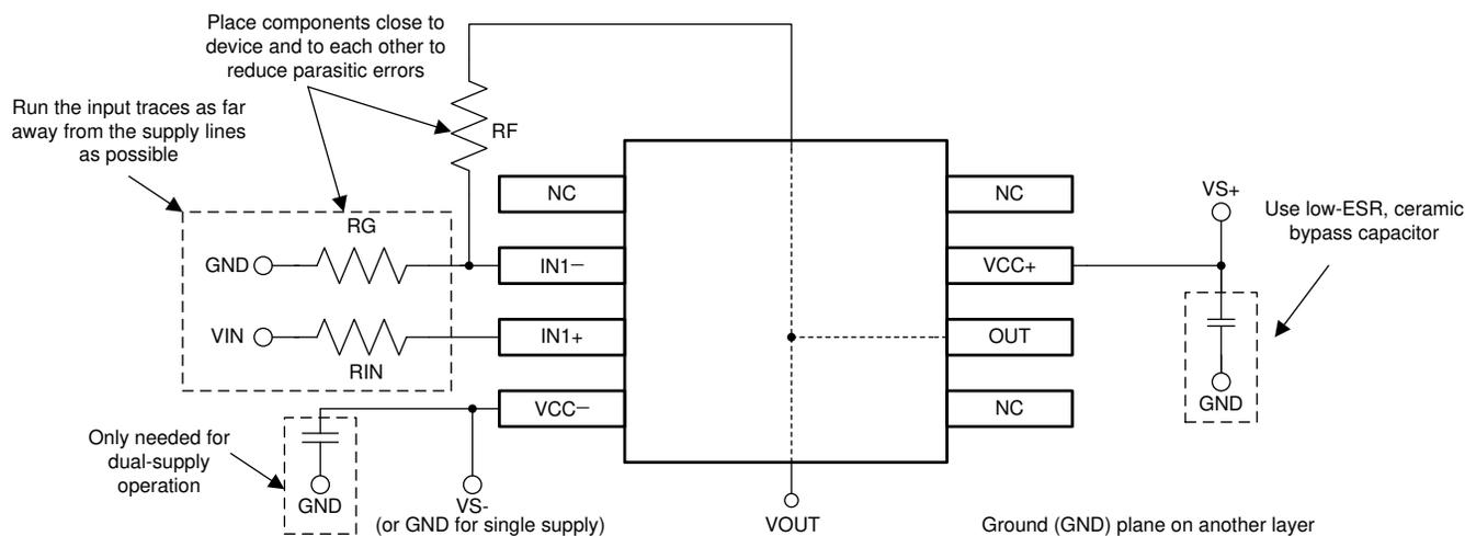
图 9-13. Operational Amplifier Board Layout for Noninverting Configuration
