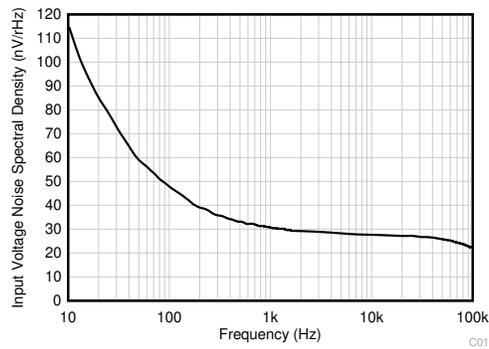
图 6-15. Equivalent Input Noise Voltage vs Frequency
