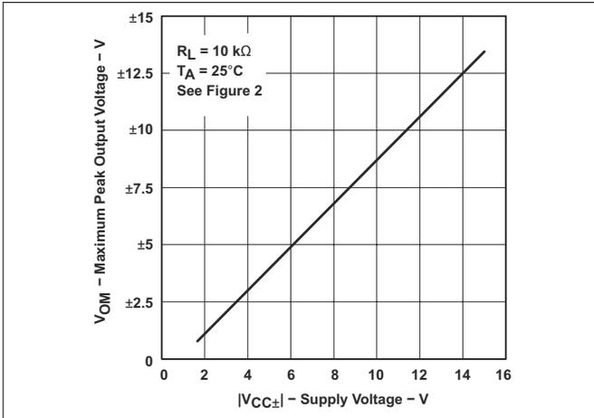
图 6-1. Maximum Peak Output Voltage vs Supply Voltage
