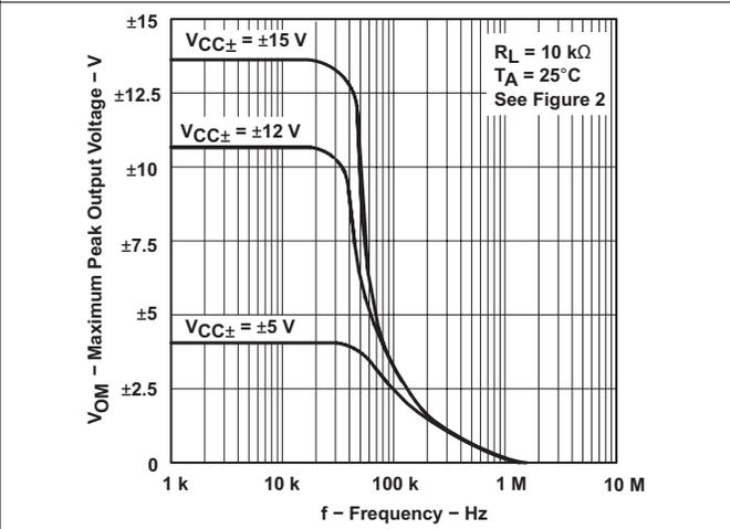
图 6-4. Maximum Peak Output Voltage vs Frequency
