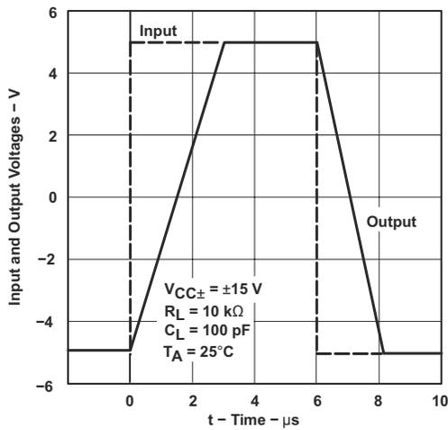
图 6-13. Voltage-Follower Large-Signal Pulse Response vs Time
