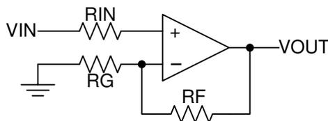
图 9-12. Operational Amplifier Schematic for Noninverting Configuration
