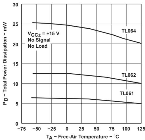
图 6-9. Total Power Dissipation vs Free-Air Temperature
