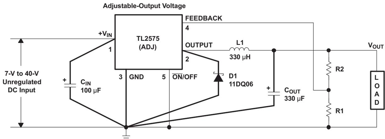
$$V_{OUT} = V_{REF} (1 + R2 / R1) = 5 V$$
