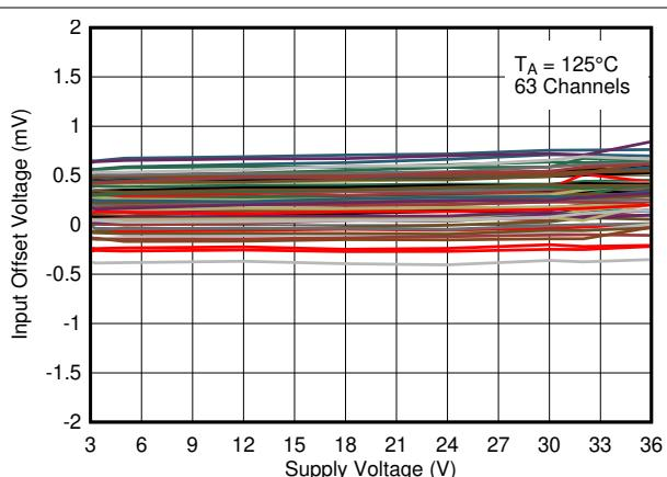
图 6-17. Input Offset Voltage vs. Supply Voltage at  $125^\circ\text{C}$
