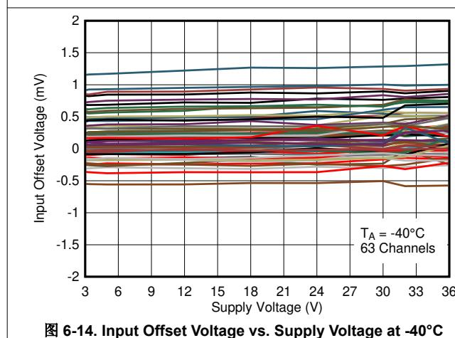
图 6-14. Input Offset Voltage vs. Supply Voltage at -40°C
