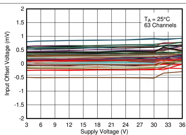
图 6-15. Input Offset Voltage vs. Supply Voltage at 25°C
