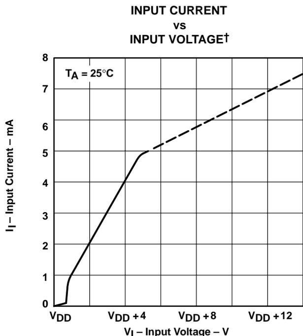
† The dashed line identifies an area of operation where some degradation of parametric performance may be experienced.
