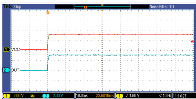
Figure 15. TMP303A Power-On Response, T_A Greater Than 60°C
