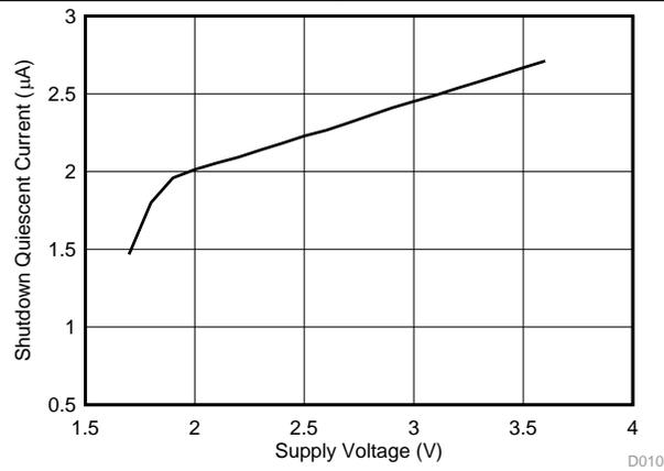
**Figure 10. Shutdown Quiescent Current vs Supply Voltage**
