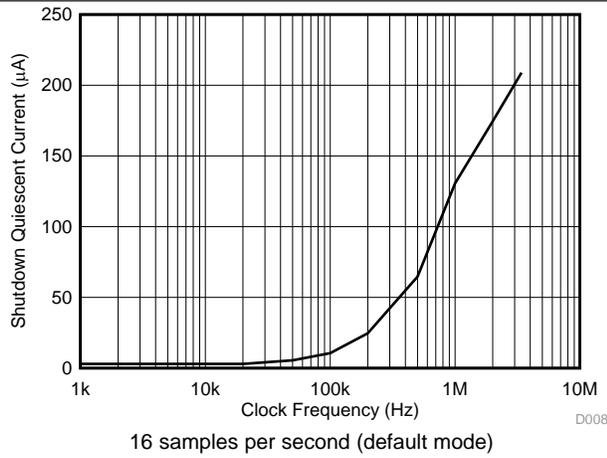
**Figure 8. Shutdown Quiescent Current vs SCL Clock Frequency**
