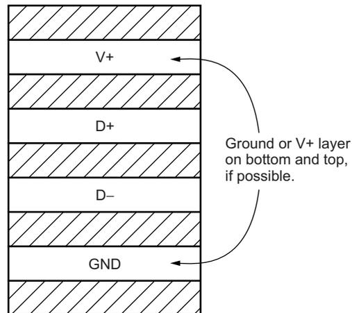
NOTE: Use a minimum of 5-mil (0.127 mm) traces with 5-mil spacing.
