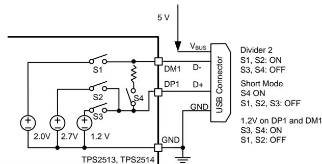
Figure 12. TPS2513 and TPS2514 DCP Auto-Detect Functional Diagram
