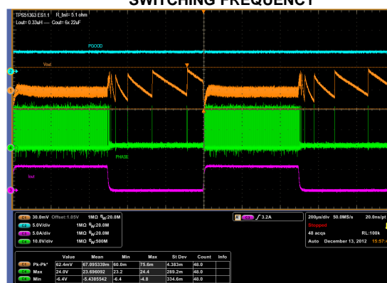
Figure 22. f = 800\text{kHz} , V_{IN} = 20\text{V} , I_{OUT} = 0-6\text{A}
