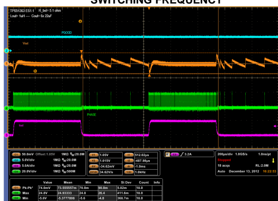
Figure 21. f = 400\text{kHz} , V_{IN} = 20\text{V} , I_{OUT} = 0-5\text{A}
