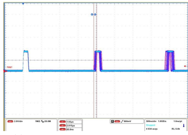
图 8-10. Steady-state PWM jitter channel A
