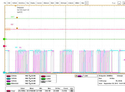
图 32. I 2 C READ (Address=31d, Cmd=0x79): ACK 0x10C8. I OC = 15 A
