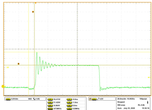
图 6-22. Switch Node Ringing and Dead-Time at 10-A Output Current
