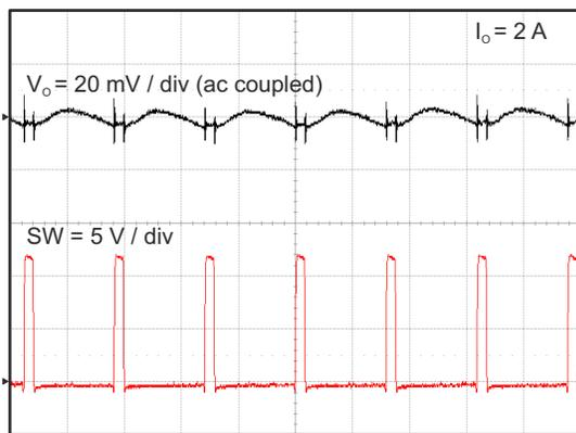
图 8-10. Tps562200 Output Voltage Ripple
