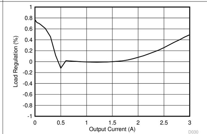
图 8-20. Tps563200 Load Regulation,  $V_I = 12\text{ V}$
