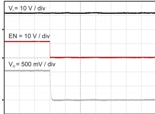
图 8-30. Tps563200 Shutdown Relative to  $EN$
