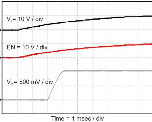
图 8-27. Tps563200 Start-up Relative to V<sub>i</sub>
