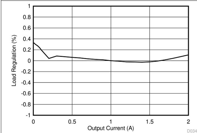
图 8-4. Tps562200 Load Regulation,  $V_I = 5\text{ V}$
