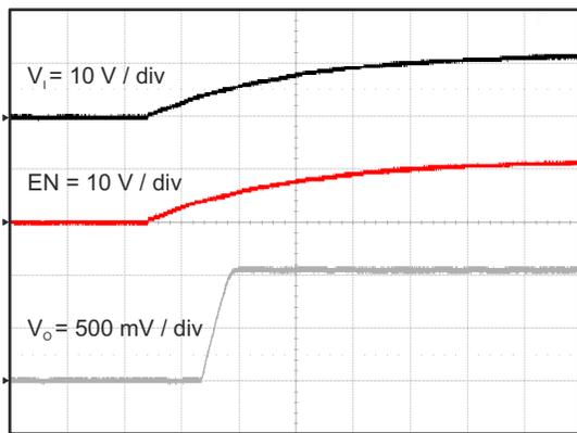
图 8-12. Tps562200 Start Up Relative to V<sub>I</sub>
