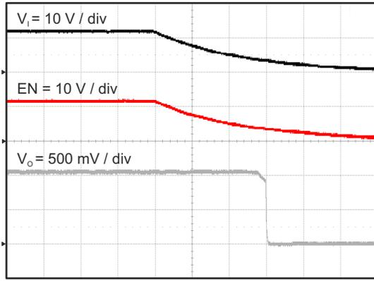
图 8-14. Tps562200 Shut Down Relative to  $V_1$
