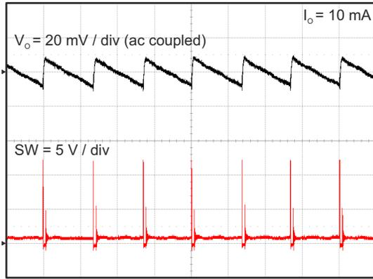
图 8-8. Tps562200 Output Voltage Ripple
