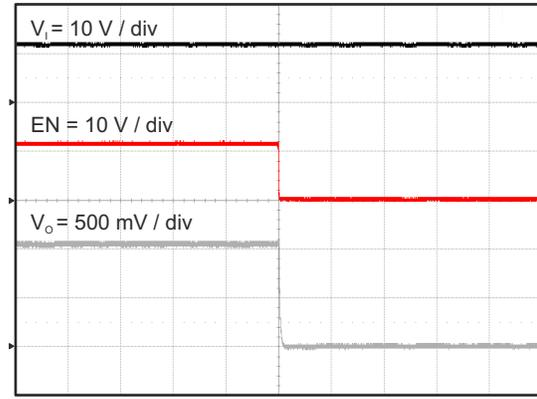
图 8-15. Tps562200 Shut Down Relative to  $EN$
