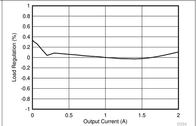
图 8-5. Tps562200 Load Regulation,  $V_I = 12\text{ V}$
