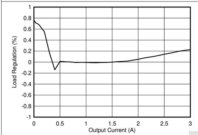
图 8-19. Tps563200 Load Regulation,  $V_I = 5\text{ V}$
