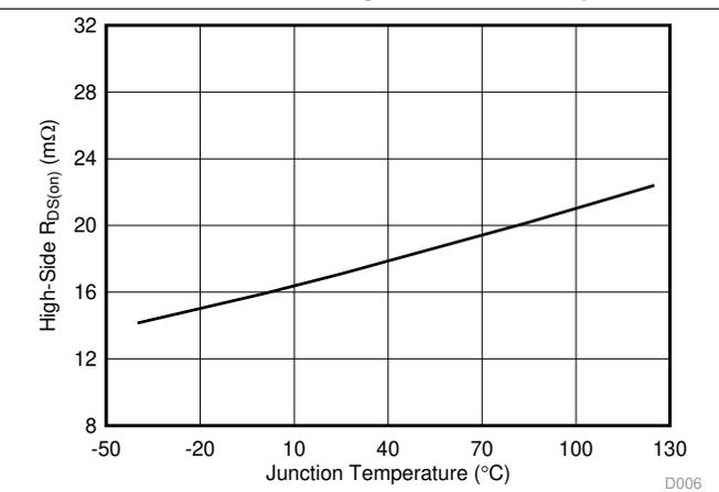
图 6. High-Side R<sub>DS(on)</sub> vs Junction Temperature
