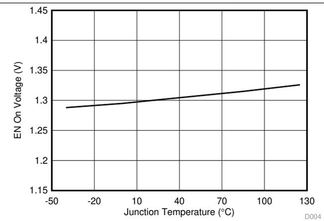
图 4. Enable On Voltage vs Junction Temperature
