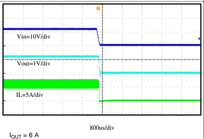
图 28. Shut Down Relative to  $V_{IN}$  Falling
