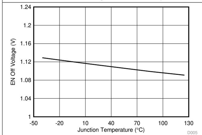
图 5. Enable Off Voltage vs Junction Temperature
