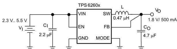
**Figure 1. Smallest Solution Size Application (Fixed Output Voltage)**
