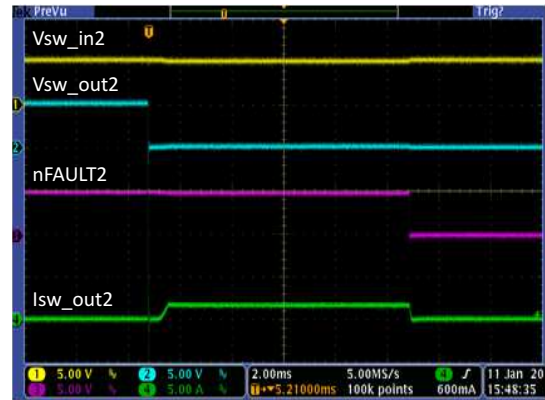
Figure 31. Power Switch2 Current Limit Operation
