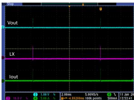
Figure 20. Buck Hiccup Response to Hard-Short Circuit
