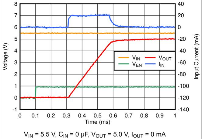
图 6-32. Startup Inrush Current With  $C_{OUT} = 1\ \mu\text{F}$
