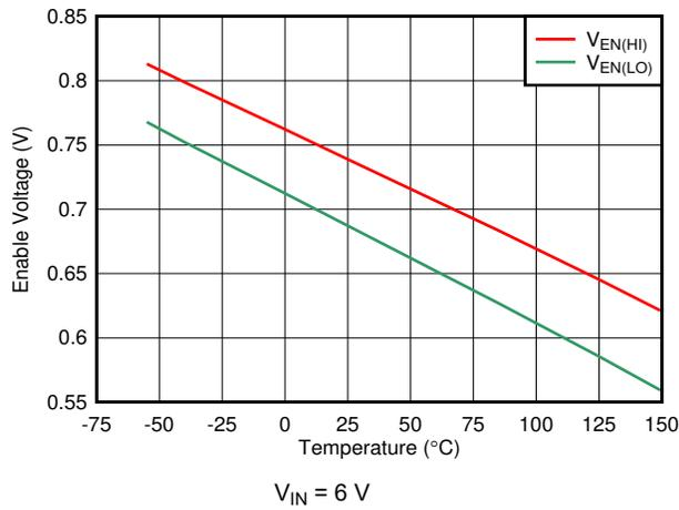
图 6-13.  $V_{EN(HI)}$  and  $V_{EN(LO)}$  Threshold vs Temperature
