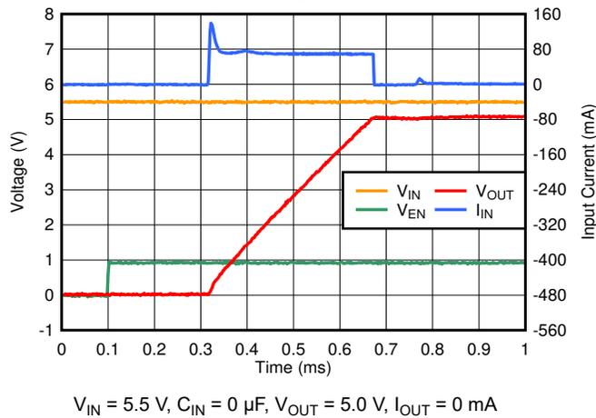
图 6-33. Startup Inrush Current With  $C_{OUT} = 4.7\ \mu\text{F}$
