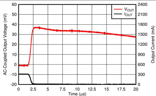
$V_{IN} = 3.8\text{ V}$ ,  $V_{OUT} = 3.3\text{ V}$ ,  $I_{OUT}$  slew rate =  $0.5\text{ A}/\mu\text{s}$
