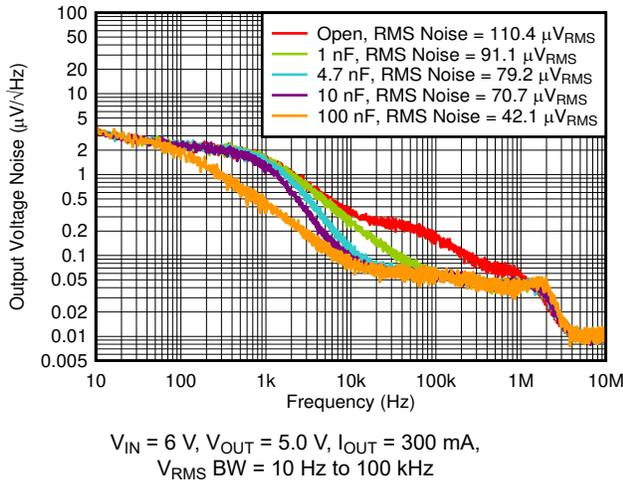
图 6-31. Output Noise vs Frequency and  $C_{FF}$
