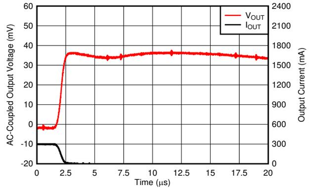
$V_{IN} = 5.5\text{ V}$ ,  $V_{OUT} = 5.0\text{ V}$ ,  $I_{OUT}$  slew rate =  $1\text{ A}/\mu\text{s}$
