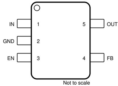
图 5-1. DBV Package, 5-Pin SOT-23, Top View
