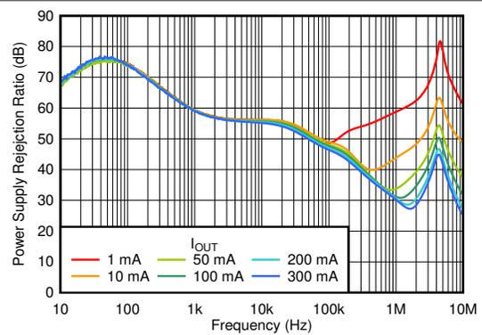
$V_{IN} = 2.2\text{ V}$ ,  $C_{IN} = 0\ \mu\text{F}$ ,  $V_{OUT} = 1.2\text{ V}$
