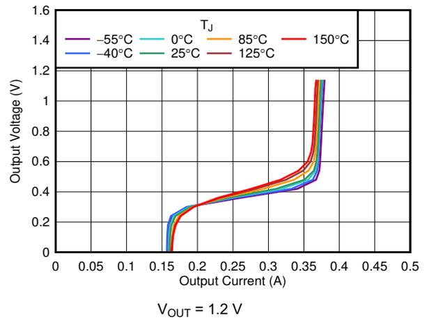
图 6-14. Foldback Current Limit vs  $I_{OUT}$  and Temperature
