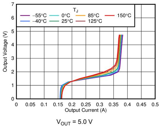
图 6-15. Foldback Current Limit vs  $I_{OUT}$  and Temperature
