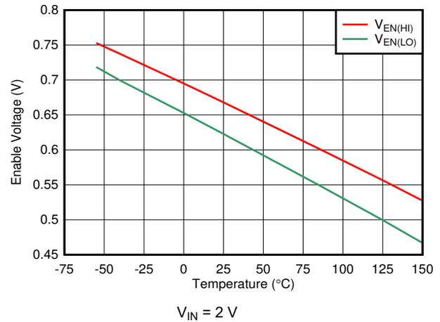
图 6-12.  $V_{EN(HI)}$  and  $V_{EV(LO)}$  Threshold vs Temperature
