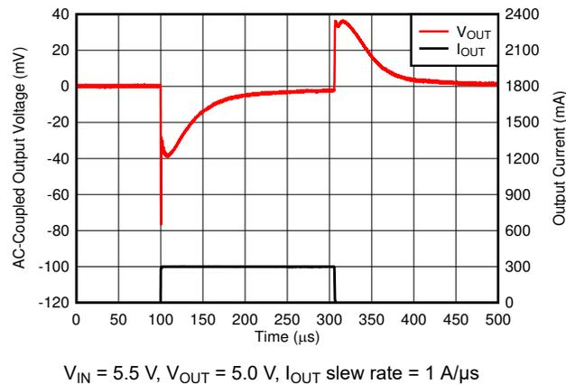
图 6-18.  $I_{OUT}$  Transient From 1 mA to 300 mA
