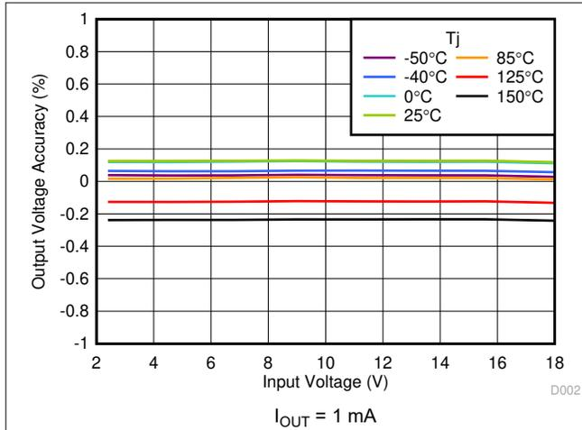
图 6-1. Line Regulation vs  $V_{IN}$
