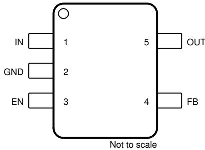
图 5-1. DBV Package (Adjustable), 5-Pin SOT-23 (Top View)
