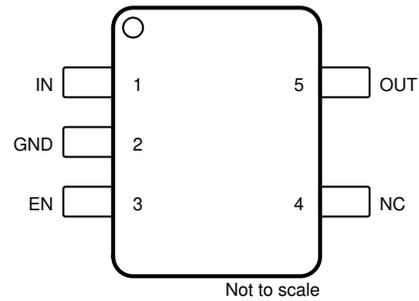
图 5-2. DBV Package (Fixed), 5-Pin SOT-23 (Top View)
